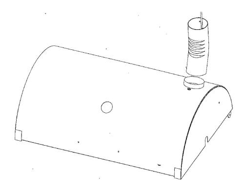
To install the temperature gauge (item #22), insert into center hole on grill lid (item #17), then turn it clockwise to upright position.
